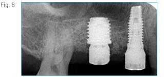
Radiograph at second-stage surgery 4 months post-op. Manual platform switching was done on the T3<sup>®</sup> Short Implant by placing a 5 mm diameter healing abutment on the 6 mm diameter implant.
